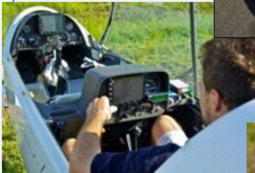
Instrument Panels for Chad (pilot) and a copy for his passenger (owner of glider) who sits in the front seat.
