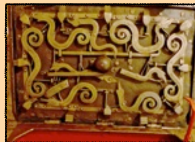
UNPICKABLE LOCK This is an example of the first type of lock mechanism made out of iron located under the lid of a money box - pretty hard to pick this lock I can tell you.
