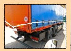
RING THE BELL Noticed a string running around this truck over the back doors. If someone tries to open them the string is tightened and a bell warns the driver.
